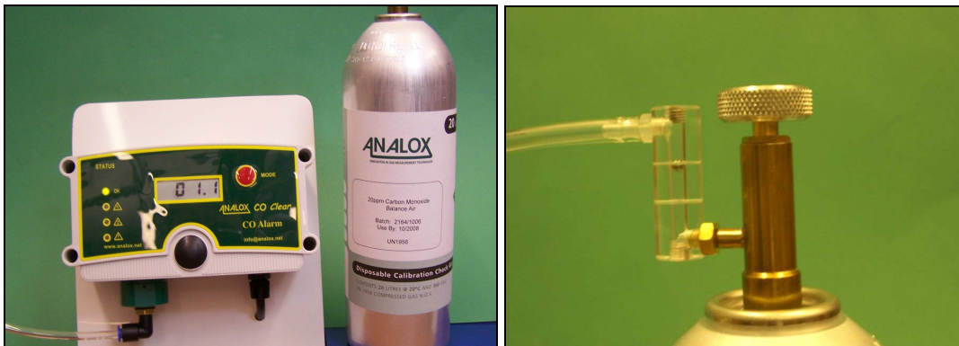
Connecting of the gas cylinder
